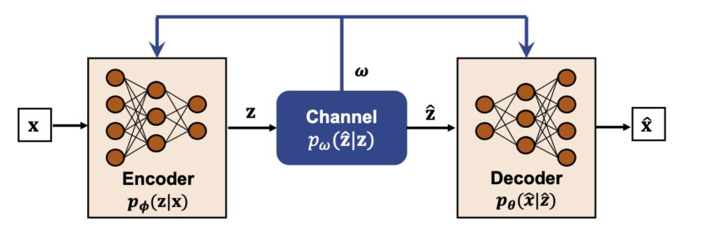
The considered system model of point-to-point communication with known channel conditions at the transmitter and receiver.
